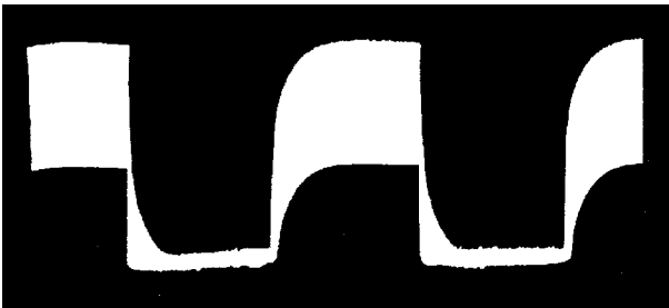
21-4 PIN diode switching using square-wave chopper waveform.
